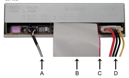
Figure 4 - 28 : Cabling an Optical Device
